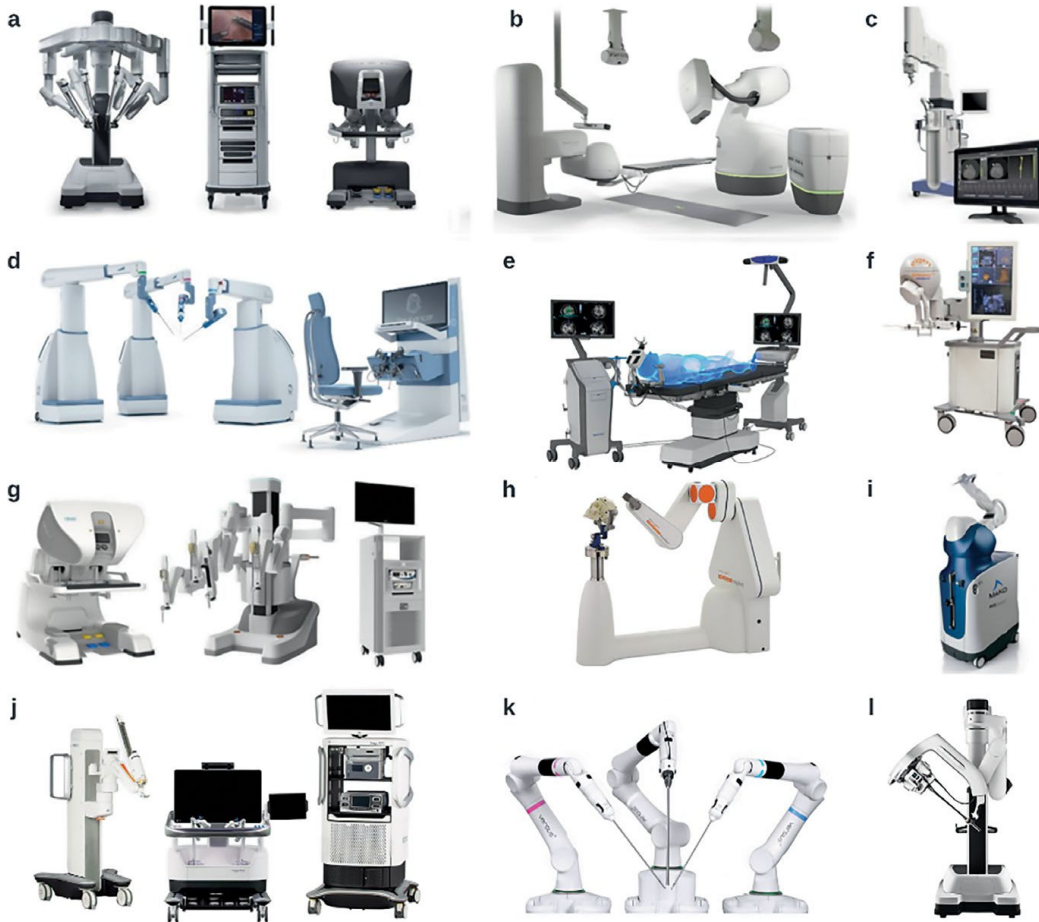
Fig. 3 Commercialized, ready-to-launch, and advanced research prototype robotic surgical systems along the three main control approaches (teleoperational, cooperative, image-guided)(a) Da Vinci Xi, (b) CyberKnife, (c) TSolution-One, (d) Senhance Surgical Robotic System, (e) iSYS/Micromate/Stealth autoguide robot, (f) Eigen ARTEMIS, (g) Revo-i, (h) Neuromate, (i) Mako, (j) Hugo RAS system, (k) Versius, (l) da Vinci SP
