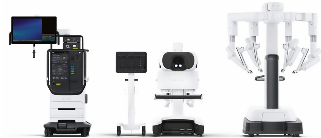
Fig. 4 The 2024 version, generation 5 of the da Vinci surgical system. It features improved accuracy and precision, advanced force sensing, expanded computing power and advanced data capabilities, complete workflow support, and greater surgeon comfort. (Image: courtesy of Intuitive)
