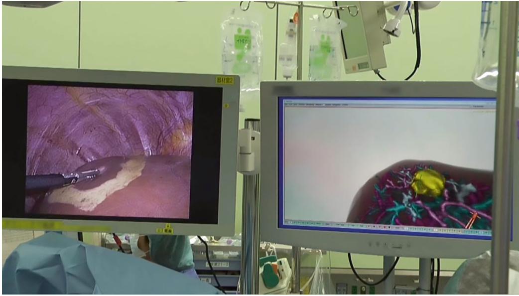
Fig. 3 Surgical navigation during laparoscopic hepatectomy. The right and left monitors display the surgical assistance image from the surgical navigation system and laparoscopic image from the laparoscope, respectively. The brown, yellow, purple, and blue regions in the surgical assistance image indicate the liver, tumor, portal vein, and hepatic vein, respectively
